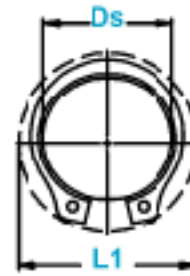
Clearance Diameter Expanded Over Shaft
