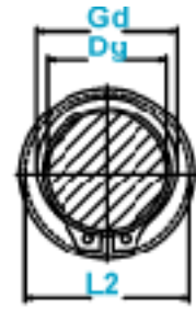
Clearance Diameter & Gaging Diameter Released in Groove
