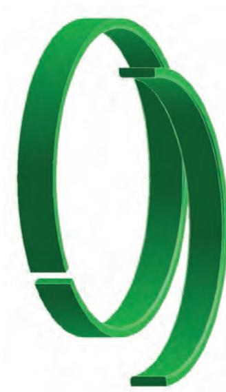
WPT profile tight-tolerance piston wear rings are the premier bearings for light- to heavy-duty hydraulic applications. WPT profile wear rings are available in standard sizes from 1" up to 12" bore diameters (larger sizes upon request). WPT profile wear rings feature chamfered corners on the I.D. and are designed to snap closed during assembly to hold tight against the piston, eliminating bore interference and simplifying installation.
