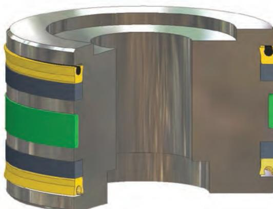
*MB installed in Piston Gland*
