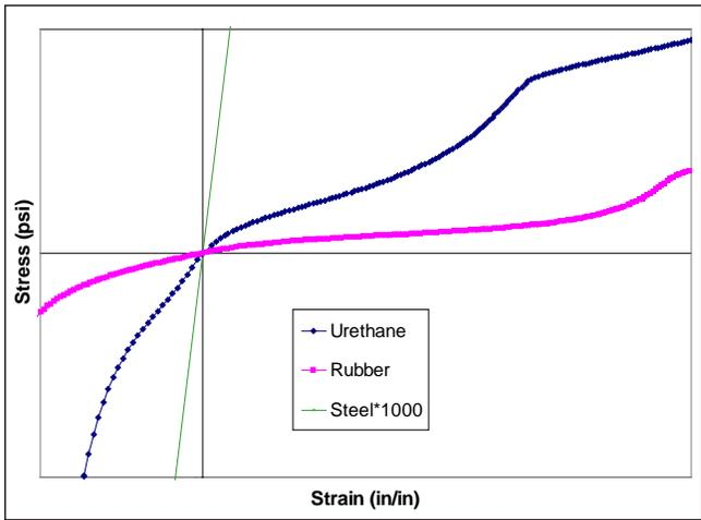
Figure 2-26. Stress/Strain relationship of steel vs. elastomers
