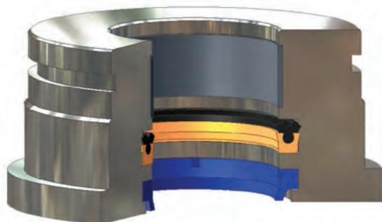
SL installed in Rod Gland
