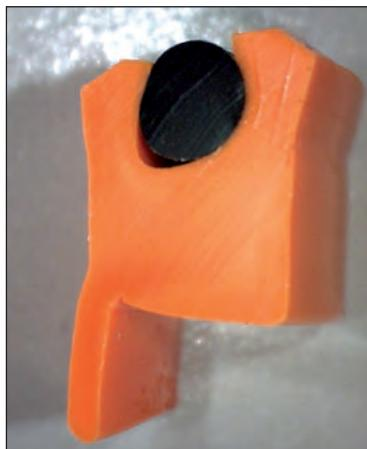
Figure 2-5. Extrusion damage
