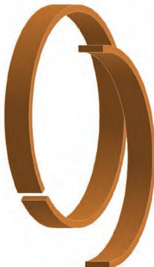
PDT profile wear strip is available in a variety of PTFE blends and provides excellent low-friction performance in pneumatics and light-duty hydraulics. PDT profile wear strip is available in cut-to-length versions as well as bulk strip. Cut-to-length part numbers reduce prep time by providing precision end cuts and ready-to-install diameters. Bulk strip offers versatility and reduces part number inventory by providing universal sizing in one part number.
