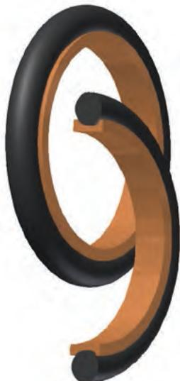
The Parker CR profile is a cap seal with anti-extrusion, low friction and low wear features. The seal is a bi-directional rod seal for use in pneumatic and low to medium duty applications. Because of its short assembly length, it requires minimal space in the rod housing. The three CR profiles will fit into standard o-ring grooves without modification. Parker's CR profiles will retrofit non-Parker seals of similar design.
