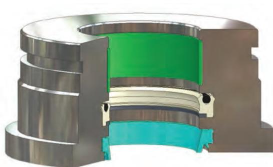
PAB Profile installed in Rod Gland
