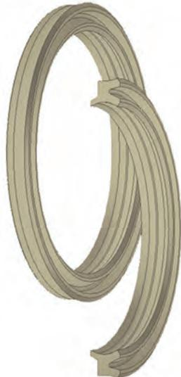
The AY profile can be used as a heavy to light duty wiper. When used in high pressure applications with the proper Parker rod seals, the AY complements the sealing system by providing an additional beveled sealing lip, yielding excellent film-breaking and the driest rod sealing available. These dual acting features also enable it to be used by itself in low pressure applications as both the rod seal and the wiper. Knife-trimmed sealing lips ensure the best possible film breaking.
