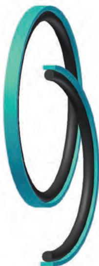
The Parker OA profile is a bi-directional piston seal for use in pneumatic and low- to medium-duty hydraulic applications. The OA profile is a two piece design utilizing a rectangular PTFE cap and standard size o-ring. The OA profile is an excellent choice for applications requiring a compact design. The unique properties of the modified PTFE provide added wear resistance for improved cycle life. Parker's OA profile will retrofit non-Parker seals of similar design.
