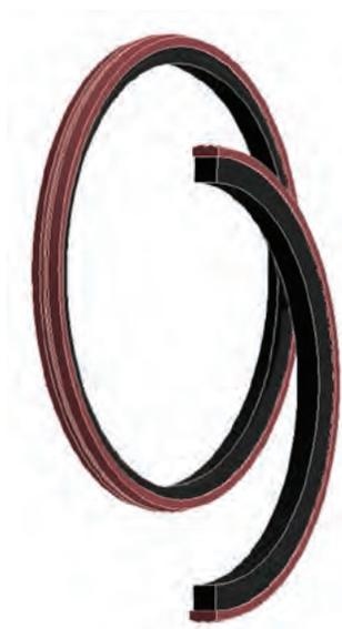
Parker's metric BP profile is a double-acting, squeeze type, piston seal for use in medium to heavy duty hydraulic applications. The standard material combination for the profile's components are a TPU cap in Resilon® 4304 polyurethane with improved sliding and high modulus, and a rectangular cross-section NBR elastomer energizer. The BP profile is easy to install on a single part piston. The unique cap design of the BP profile makes the seal insensitive to pressure spikes.
