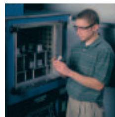
In-house fuel permeation testing paves the way for production of next-generation fuel system sealing components.
