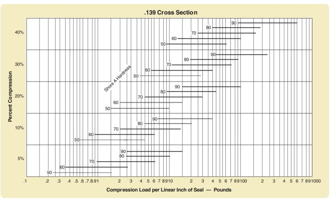
Figure 2-6: .139 Cross Section
