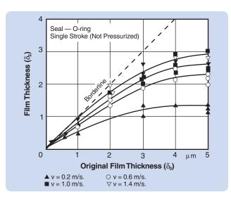
Figure 5-15: Change in Original Film Thickness as a Function of Running Speed During a Single Stroke (Border Line  $\Delta$ Theoretical maximum Values)
