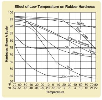
Figure 2-18: Effect of Low Temperature on Rubber Hardness
