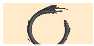
Figure 10-2: Extruded O-Ring
