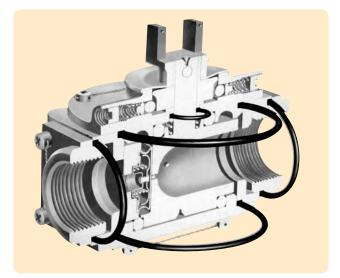
Figure 1-8: Static Seal Application
