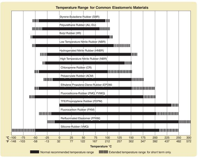
Figure 2-3: Temperature Range for Common Elastomeric Materials
