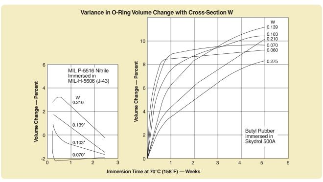
Figure 2-30: Variance in O-ring Volume Change With Cross-Section W \*Averages of many samples
