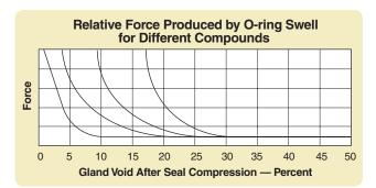
Figure 2-20: Relative Force Produced by O-ring Swell
