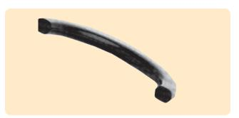
Figure 10-1: Characteristic compression set — high deformation -seen as flattening on all contact surfaces.
