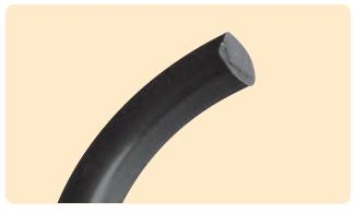
Figure 10-5: Wear is Seen as Flattening of O-ring on One Side
