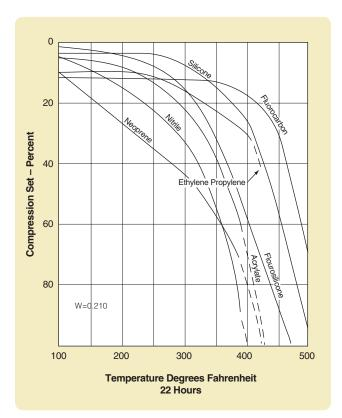
Figure 2-16: Compression Set .210 Cross Section
