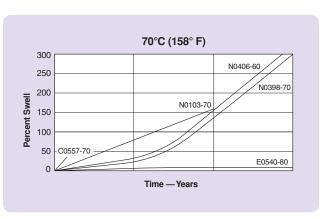
Figure 3-13: Water and Steam Resistance at 70°C (158°F)
