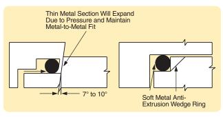
Figure 6-2: Clearance Control for High Pressure Seals
