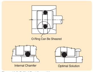
Figure 10-7: Drilled Port Assembly
