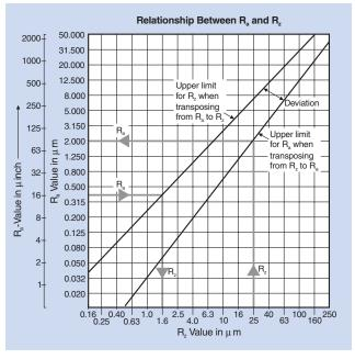
Figure 5-5: Relationship Between  $R_{\text{a}}$  and  $R_{\text{z}}$
