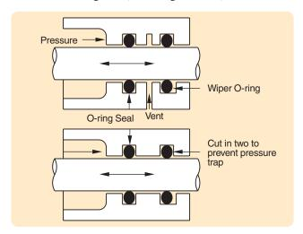
Figure 1-14: Wiper Installation
