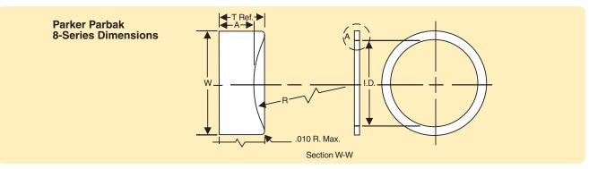
Parker Parbaks were developed primarily for service in petroleum based hydraulic fluids, at -4°C to 121°C (-40°F to 250°F). Parker's standard Parbak compound N1444-90, provides the maximum benefits in back-up ring service. Compounds for use in other fluids and for temperatures up to 204°C (400°F) are available upon request.
