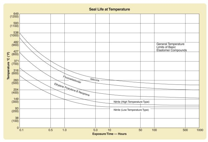
Figure 2-28: Seal Life at Temperature
