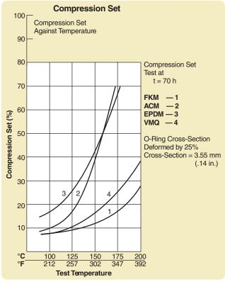
Figure 2-13: Compression Set vs. Polymer Family
