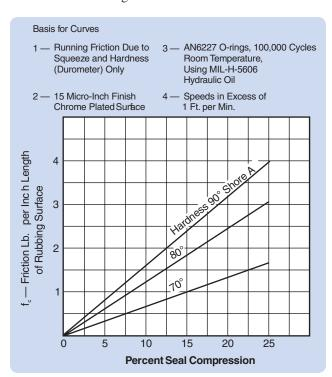
Figure 5-9: Friction Due to O-ring Compression
