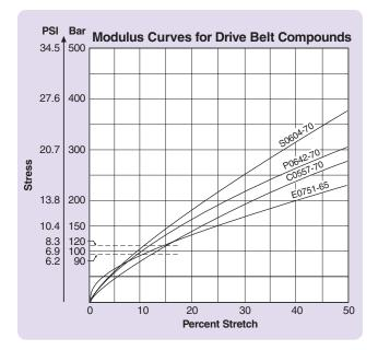
Figure 3-14: Modulus Curves for Drive Belt Compounds
