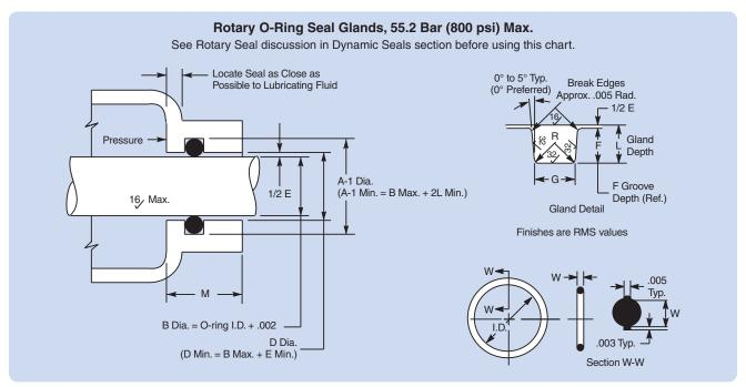
Note: Due to effect of centrifugal force, do not locate groove in shaft. Refer to Design Chart 5-4 (below) and Design Table 5-4 for dimensions.
