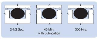
Figure 5-8: Flow of O-Ring into Metallic Surfaces
