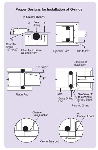
Figure 3-4: Proper Designs for Installation of O-rings
