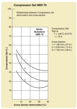
Figure 2-11: Compression Set NBR 70
