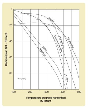
Figure 2-14: Compression Set .070 Cross Section
