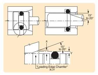
Figure 10-6: Chamfers
