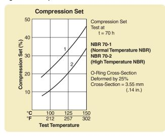
Figure 2-12: Compression Set vs. NBR 70 Compounds
