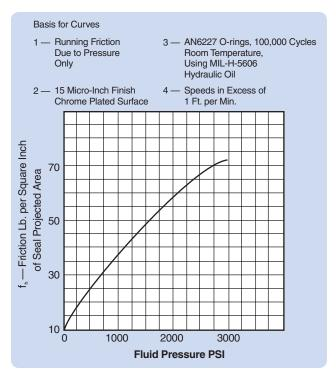
Figure 5-10: Friction Due to Fluid Pressure
