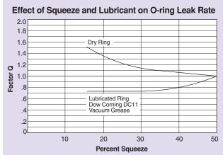
For helium leak rate, a variation of ±50% from the predicted value should be anticipated to allow for limitations in the accuracy of test equipment and available standards, and for variations between samples.
