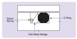
Figure 3-1: Spring-Loading for Low Temperature
