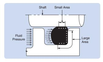
Figure 5-16: Action of Fluid Pressure to Prevent Rolling of O-ring
