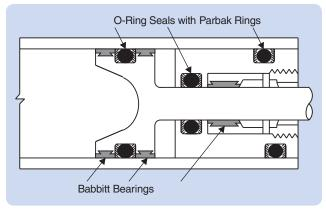
Figure 5-1: O-ring Seals with Bearings
