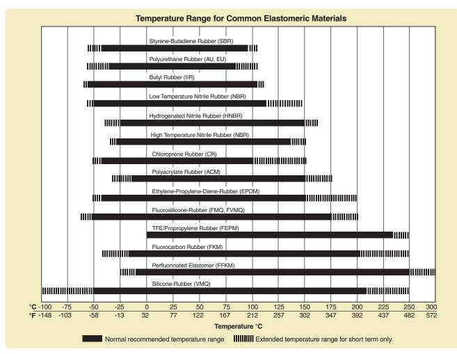
Figure 2-25: Temperature Capabilities of Principal Elastomers Employed in Seals
