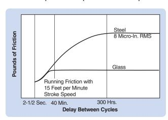
Figure 5-7: Change of O-ring Friction with Time at Rest
