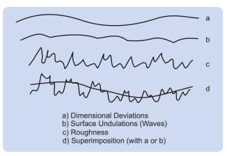
Figure 5-3: Surface Finish Structure
