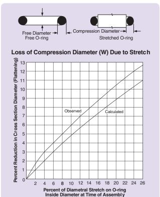
The "observed" curve is reproduced by courtesy of the Research Laboratories of General Motors Corporation at the General Motors Technical Center in Warren, Michigan. This curve is based on a statistical analysis of a much larger volume of experimental data than has been available previously.
