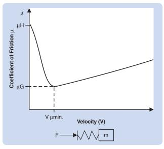
Figure 5-14: System Diagram for Stick-Slip Effect
