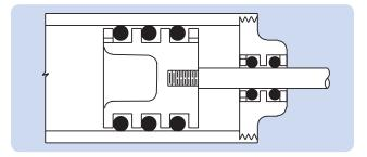
Figure 5-20: Use of Multiple O-Rings in a Floating O-Ring
