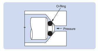
Figure 5-22: Valve Seat Seal, Standard Groove
