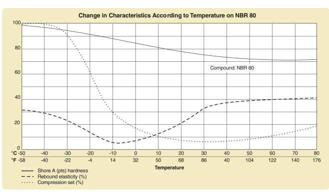
Figure 2-27: Change in Characteristics According to Temperature on NBR 80
