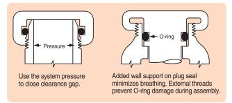
Figure 4-1: End Cap Seal
