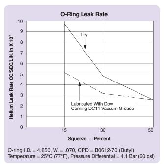
Figure 3-8: O-ring Leak Rate
