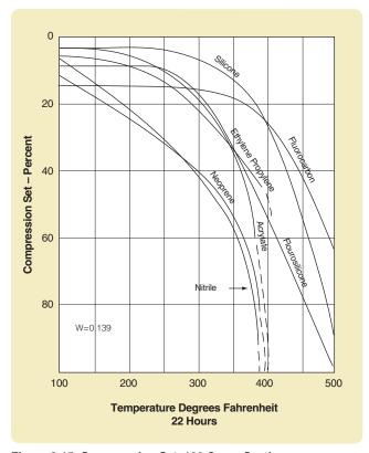
Figure 2-15: Compression Set .139 Cross Section
