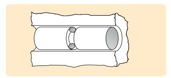
Figure 1-3: Gland and O-Ring Seal
