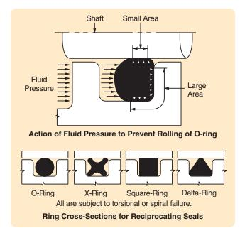
Figure 10-8: Rolling of O-ring
