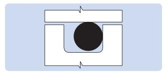
Figure 5-19: Floating O-Ring Seal
