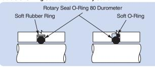
Figure 5-21: Spring-Loading for Rotary Seal
