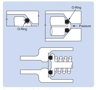
Figure 5-24: Groove Designs to Prevent Blow-Out
