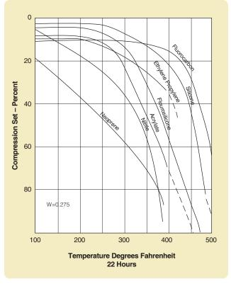
Figure 2-17: Compression Set .275 Cross Section
