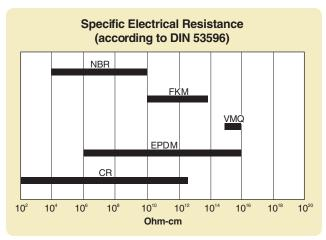
Figure 2-19: Specific Electrical Resistance (According to DIN 53596)
