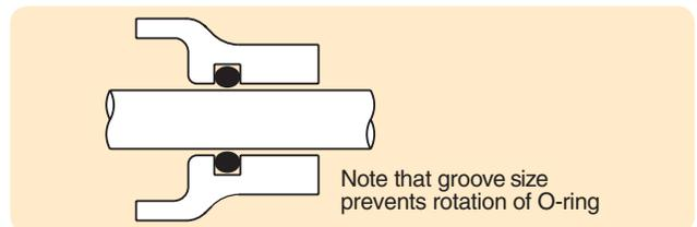
Figure 1-11: Rotary Seal
