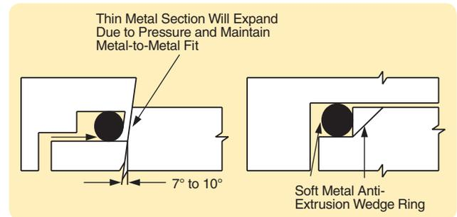
Figure 6-2: Clearance Control for High Pressure Seals
