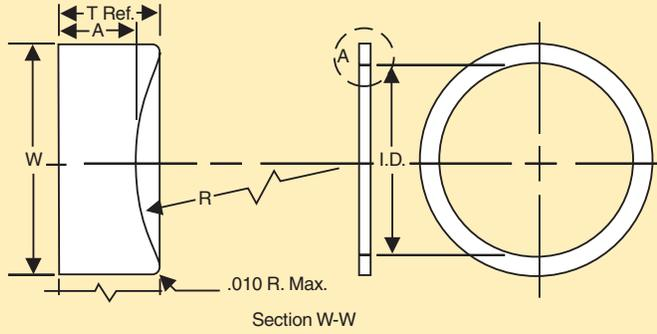
Parker Parbaks were developed primarily for service in petroleum based hydraulic fluids, at -4°C to 121°C (-40°F to 250°F). Parker's standard Parbak compound N1444-90, provides the maximum benefits in back-up ring service. Compounds for use in other fluids and for temperatures up to 204°C (400°F) are available upon request.
