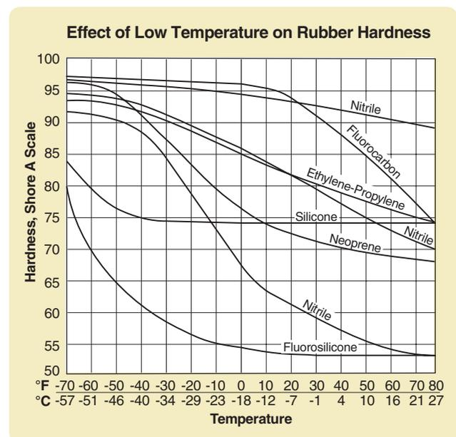
Figure 2-18: Effect of Low Temperature on Rubber Hardness
