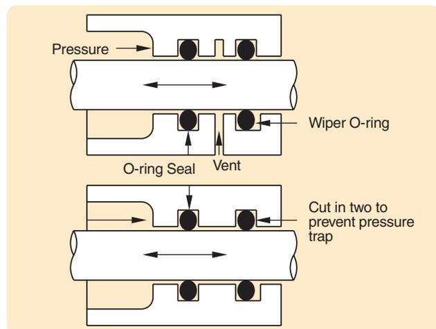
Figure 1-14: Wiper Installation
