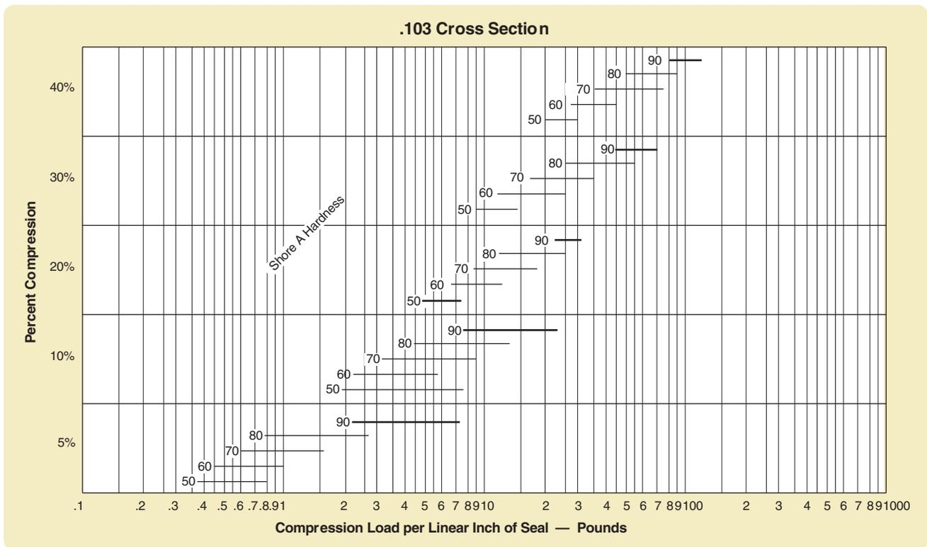
Figure 2-5: .103 Cross Section
