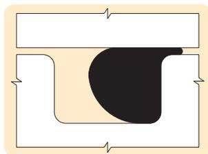
Figure 1-6: O-Ring Extruding
