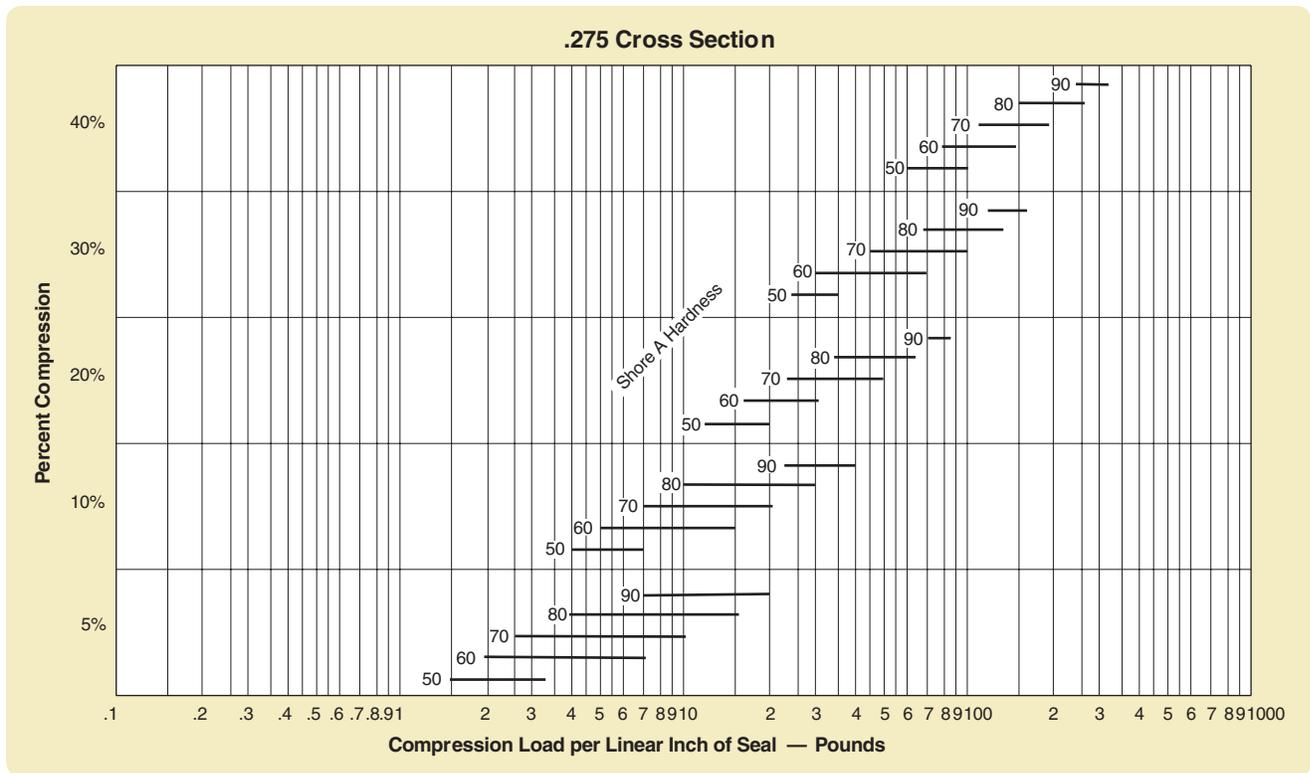
Figure 2-8: .275 Cross Section
