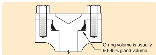
Figure 1-13: Crush Installation
