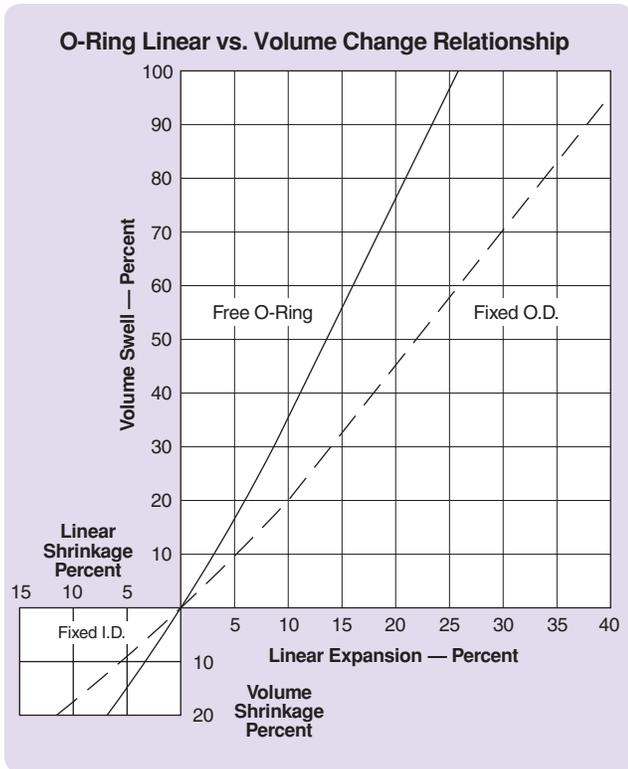
Figure 3-6: O-ring Linear vs. Volume Change Relationship
