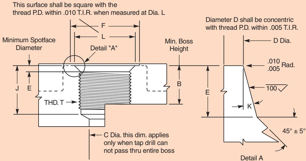
Finished tapered counterbore (Detail A) shall be free from longitudinal and spiral tool marks. Annular tool marks up to 100 micro-inches maximum will be permissible.
