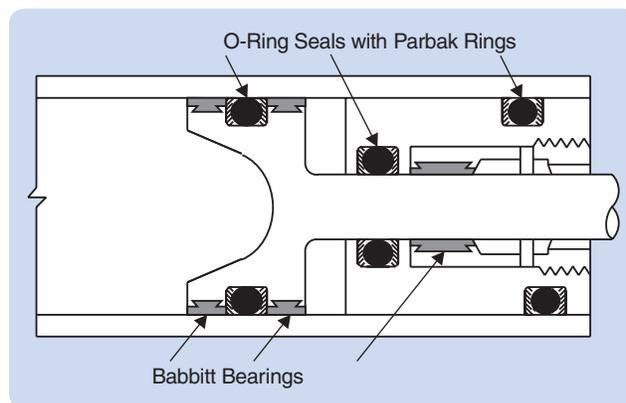
Figure 5-1: O-ring Seals with Bearings
