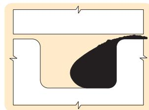
Figure 1-7: O-Ring Failure
