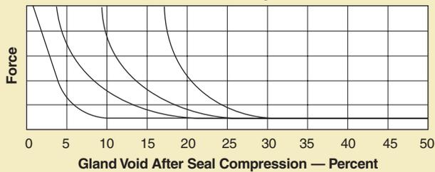
**Figure 2-20: Relative Force Produced by O-ring Swell**
