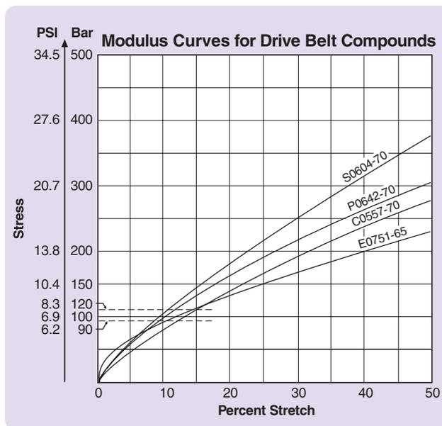
Figure 3-14: Modulus Curves for Drive Belt Compounds
