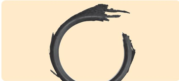
Figure 10-2: Extruded O-Ring
