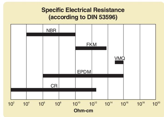
Figure 2-19: Specific Electrical Resistance (According to DIN 53596)
