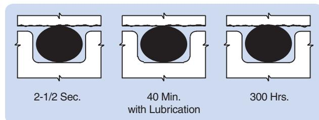
Figure 5-8: Flow of O-Ring into Metallic Surfaces
