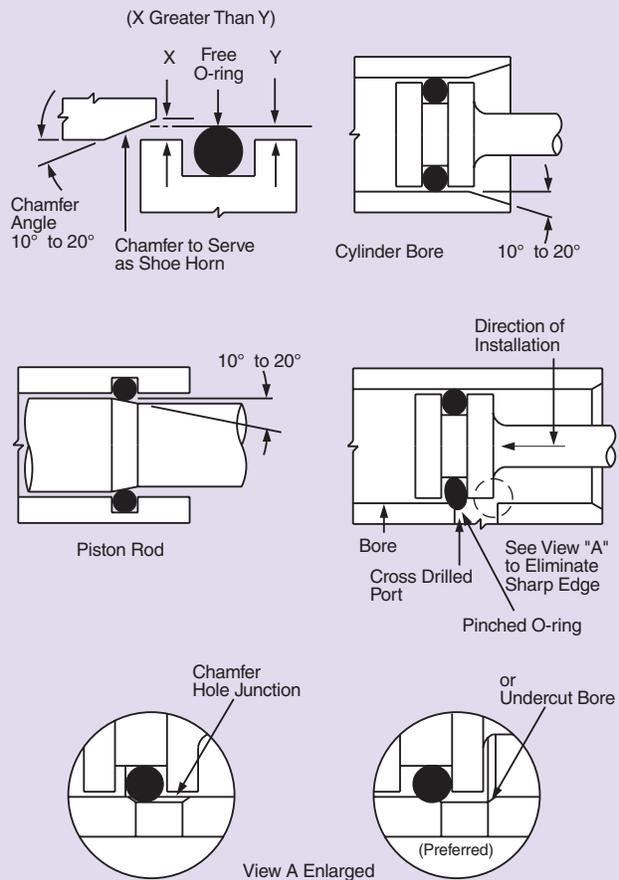
Figure 3-4: Proper Designs for Installation of O-rings
