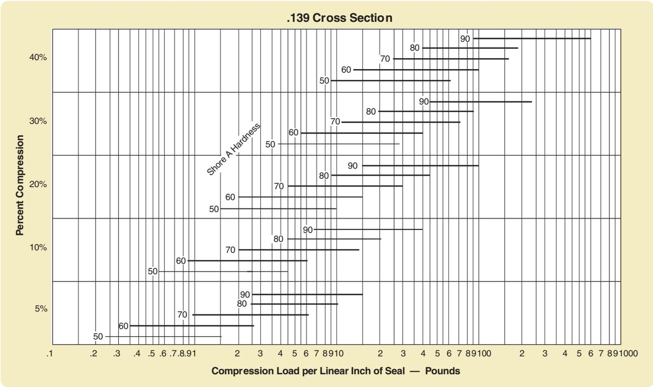
Figure 2-6: .139 Cross Section
