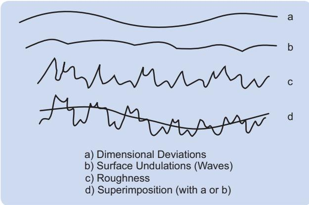
Figure 5-3: Surface Finish Structure
