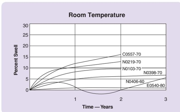
Figure 3-12: Water and Steam Resistance at Room Temperature
