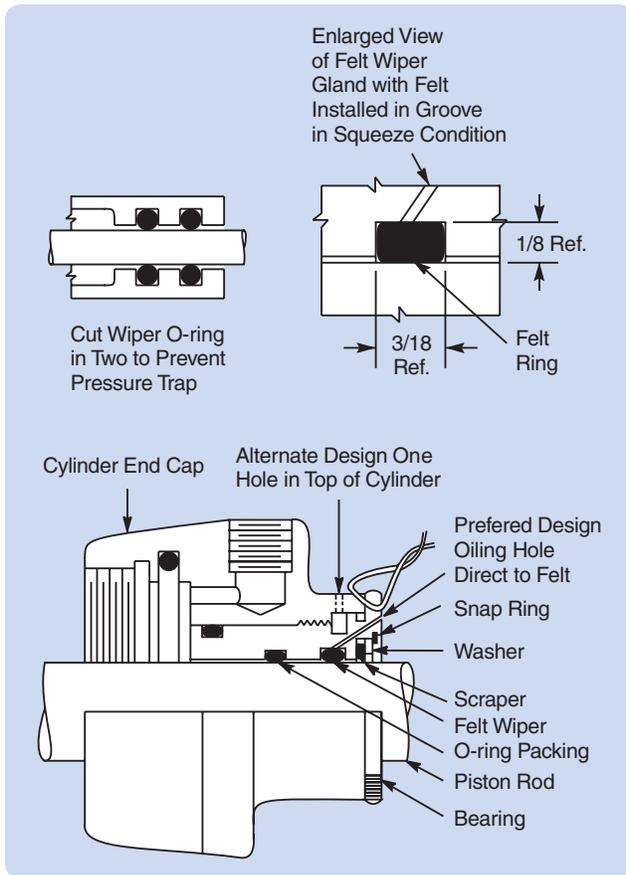
Figure 5-2: Lubrication Between Scraper and Seal Rings
