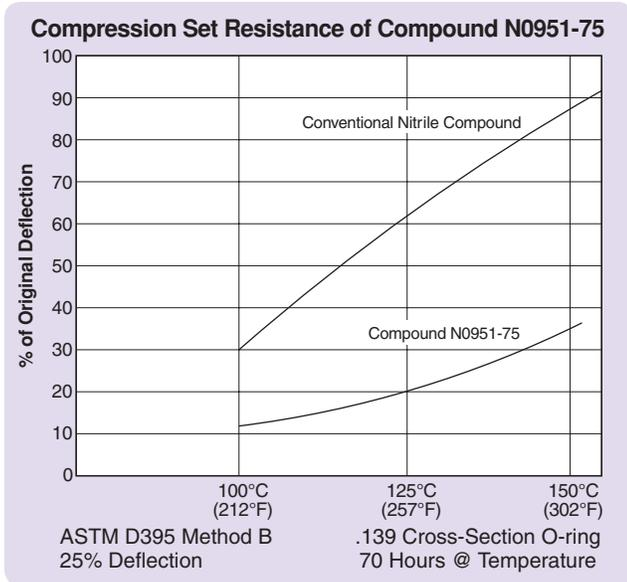
Figure 3-7: Compression Set Resistance of Compound N0951-75
