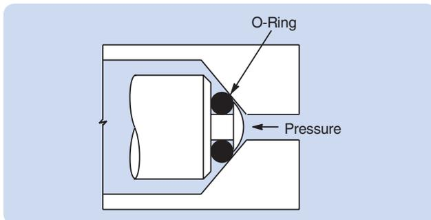
Figure 5-22: Valve Seat Seal, Standard Groove
