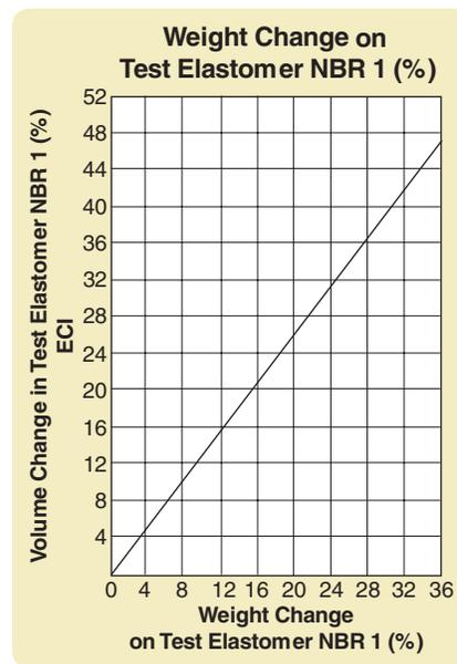
Figure 2-24: Weight Change on Test Elastomer NBR 1 (%)
