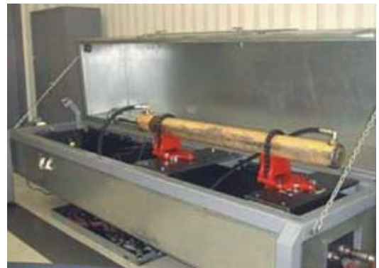
High pressure hydraulic leakage testing
