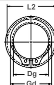
Clearance Diameter & Gaging Diameter Released in Groove.
