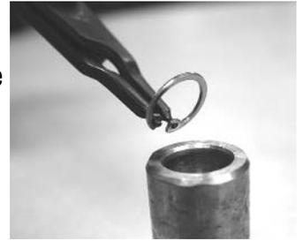
**Applicators**—Used to install radial retaining rings onto a shaft.
