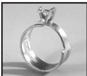
This unique, patented version of a preopened clamp is held in the open position by compressing the tangs and allowing the stop to hook on to a complementary notch on the side of one of the tangs.
