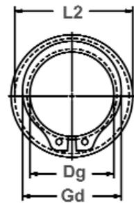
Clearance Diameter & Gaging Diameter Released in Groove.
