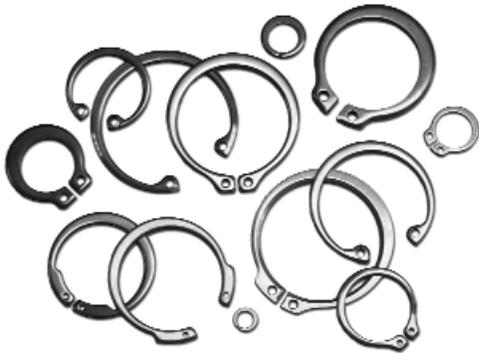
2. **Axial or Radial assembly** - Internal rings are used to position and secure parts in bores and housings. They are always installed in an axial direction. External rings hold parts on shafts, studs and similar devices and can be installed in both axial and radial directions.
