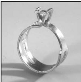
This unique, patented version of a preopened clamp is held in the open position by compressing the tangs and allowing the stop to hook on to a complementary notch on the side on one of the tangs.
