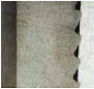
Anchorage due to plug sleeve serrations
