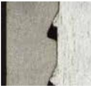
Anchorage due to plug sleeve serrations
