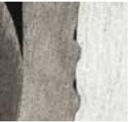
Anchorage due to plug sleeve serrations
