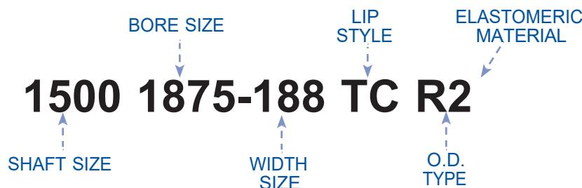
**Shaft Size** - The first four digits in the part number describe the nominal shaft size to three decimal places. If the shaft size is greater than 10 inches, five digits will be used for this portion of the part number.
