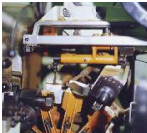
By converting to iglide® L280, the life of the bearing on this tea bag packaging machine was increased five times
