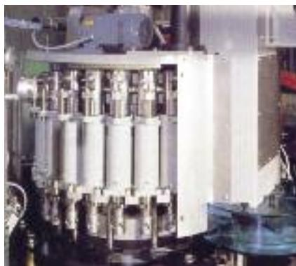
Filling applications: linear, oscillating, and rotating movements can be achieved using iglide® H370 bearings
