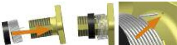
Slide the friction disc ③ and the counternut ④ over the adjusting ring. Please ensure that the adjusting ring does not rotate.
