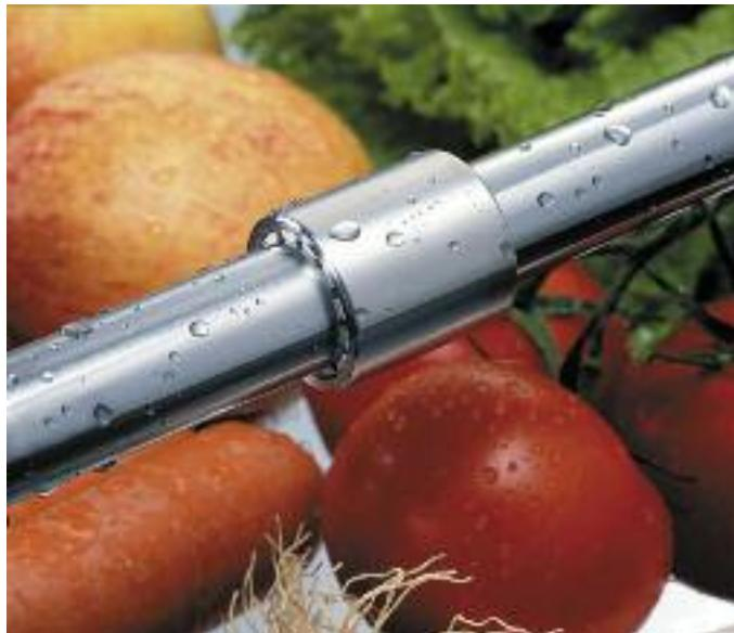
DryLin® guides and iglide® plastics are well suited for use on stainless steel shafting, and are especially good in applications requiring 300-Series stainless steels, such as 304 and 316. Since the plastic plain bearings do not have the point-to-point contact on shafting that ball bearings do, they do not require more expensive corrosion-prone case-hardened stainless steels such as 440C.
