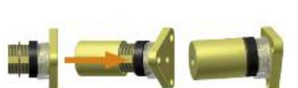
Continue to screw the adjusting ring onto the nut until the end to tension the torsion spring.
