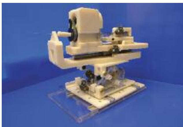
A PhD student from the Worcester Polytechnic Institute used DryLin® linear bearings and iglide® plastic bearings to facilitate motion on this MRI-guided robot, which will revolutionize the way prostate cancer is detected and treated.
