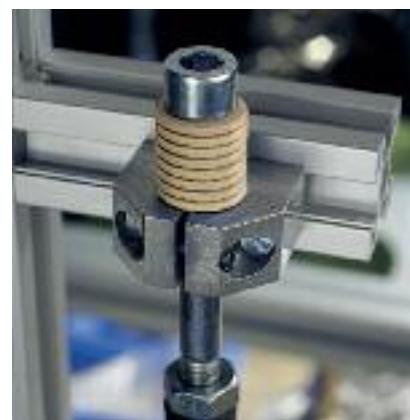
Polysorb Disc Springs in a fatigue test
