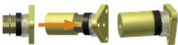
Continue to screw the adjusting ring onto the nut until the end to tension the torsion spring.
