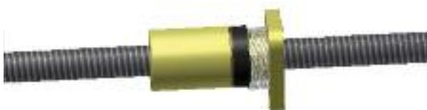
The adjusting ring can now be released. The nut will now assume a preloaded position on the lead screw.
