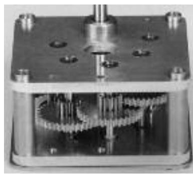
Precision mechanical gears need plain bearings with especially universal properties
