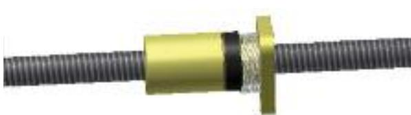
The adjusting ring can now be released. The nut will now assume a preloaded position on the lead screw.
