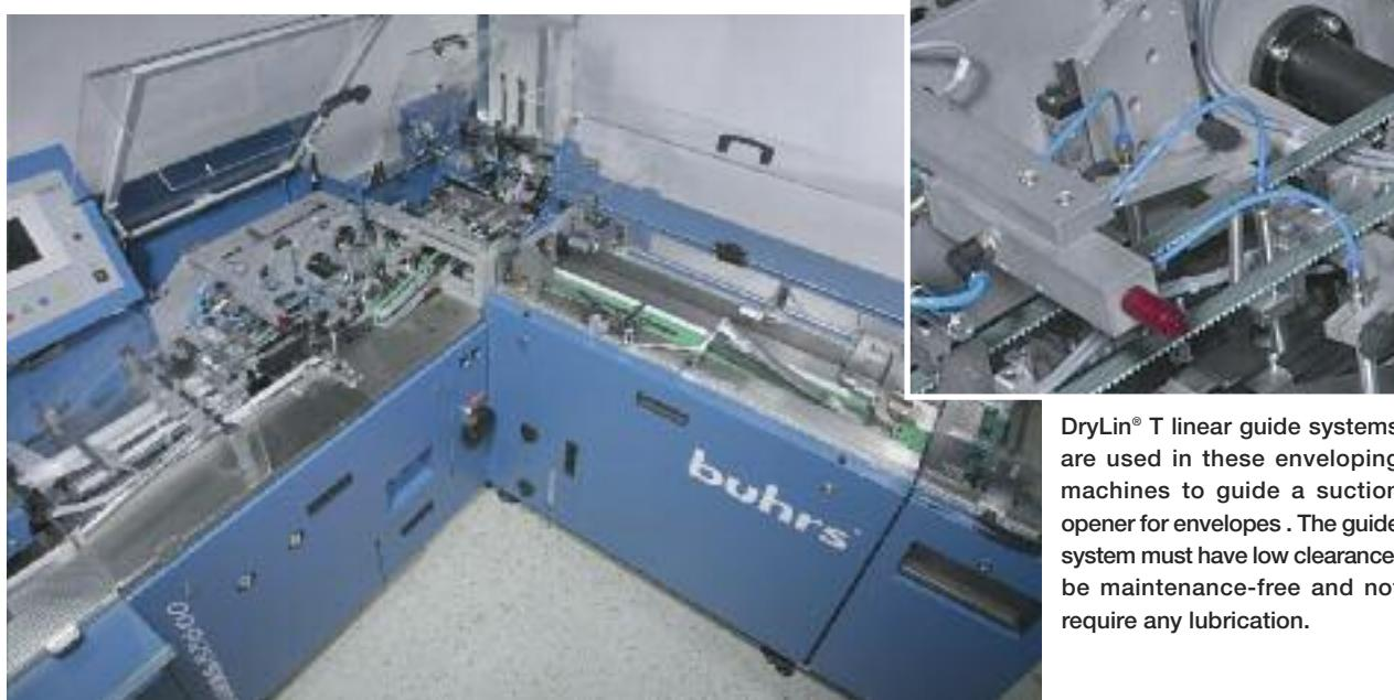
DryLin® T linear guide systems are used in these enveloping machines to guide a suction opener for envelopes. The guide system must have low clearance, be maintenance-free and not require any lubrication.
