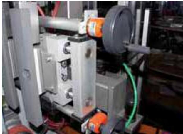
Format adjustment using DryLin® Easy Tube
